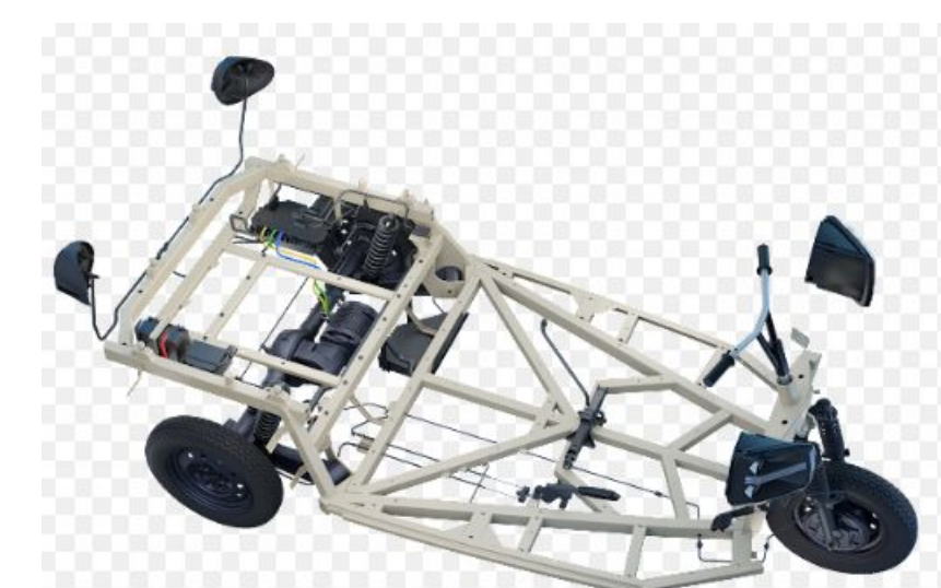
Boron steel chassis for better balance and safety
